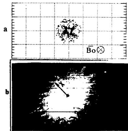
Fig. 2 Calculation data (a) and frame-photo (b, with H<sub>2</sub>-pressure ~ 0.1mT) of the plasma configuration from the point of view along magnetic field (here one large division is equal 0.1m) at time  $t \approx 1.3\text{--}1.75\mu\text{s}$ .
