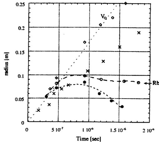
Fig. 3 Data on plasma cloud expansion in  $X, Z$  directions: -across magnetic field ( $x$  - experiment;  $\circ$  - calculation for the outer rare plasma;  $\bullet$  - calculation for plasma shell); -along field  $\diamond$  plasma front's motion according to the calculation.
