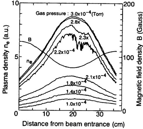
Fig. 1 Spatial distributions of the plasma density and the magnetic field density are presented. The scale of 5 on vertical axis corresponds to the density of  $1.5 \times 10^{15} \text{m}^{-3}$ . Pressure balance:  $(\epsilon E^2/2) + (\mu H^2/2) + p = \text{const.}$  is shown, where the  $p$ ,  $E$  are the plasma pressure, electric field by soliton, respectively.
