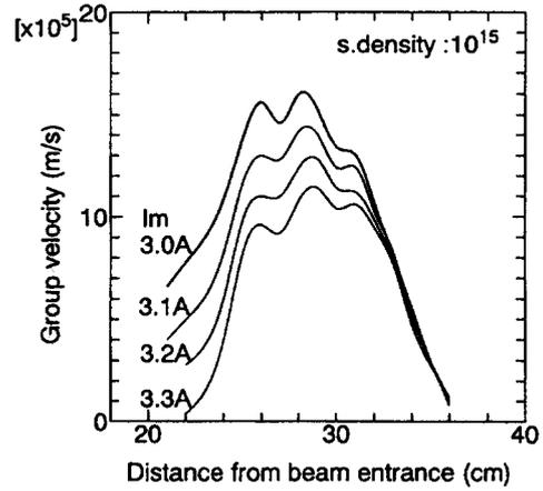
Fig. 4 Calculated group velocities from the data of fig. 1 at which main field current,  $I_m$ , is 3A, are presented as the function of position. The generated wave at 36cm point propagate oppositely against the beam, and their group velocity lessen near the position of cavities. Possible mechanism of energy accumulation of the soliton may thus be occurred by this slowing down.
