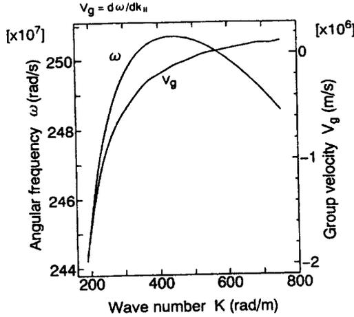
Fig. 3 Group velocity dispersion at 36cm point is presented. The region of the negative group velocity shows abnormal dispersion and the burst-wave generation is expected as in the optical solitons in fibers. We assumed that the momentum of an elementary excitation,  $\hbar k$ , is conserved at any position.
