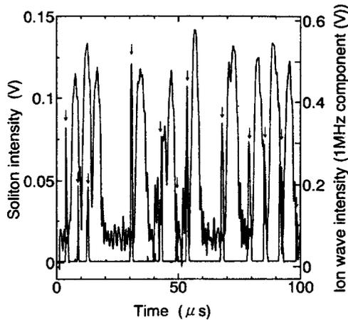
Fig. 5 The strong couplings between the soliton and the ion wave are presented. The pointed peaks shown by the arrows represent envelope solitons and wide peaks are 1MHz component of ion waves. The ion waves are surrounded by dispersive waves whose width are almost same as that of solitons.
