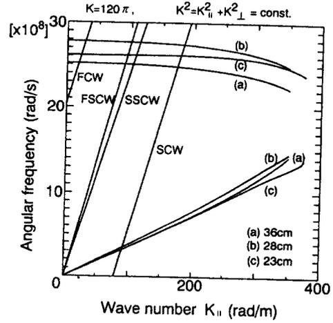
Fig. 2 Examples of dispersion relation for hybrid wave at several point are shown. The burst-wave generation by non-convective interaction between the wave branch (a) and the beam's space charge wave (SSCW) can be expected.
