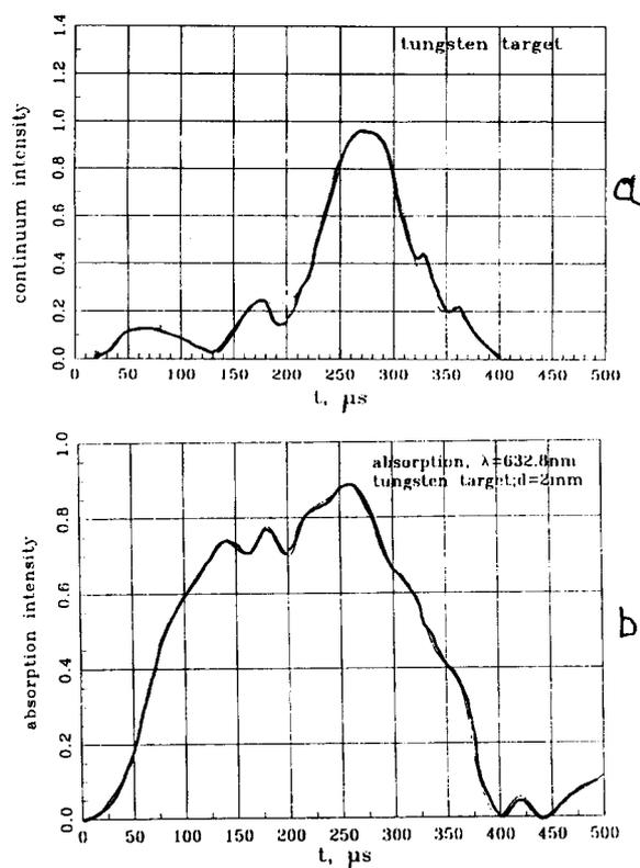
Fig. 3 a, b. The dynamics of the continuum (a) and absorption (b) intensities. Target - tungsten. Irradiation power  $P_{irr} \sim 5 \text{ MW/cm}^2$ .
