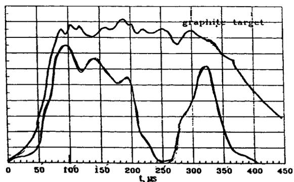
Fig. 4 The dynamics of the relative radiation intensities for two directions of registration. Target - graphite. Irradiation power  $P_{irr} \sim 5 \text{ MW/cm}^2$ . bottom curve - CIII carbon line ( $\lambda = 229.7 \text{ nm}$ ), side-on registration; upper curve - CII resonance line ( $\lambda = 426.7 \text{ nm}$ ), registration through the hole in the target.
