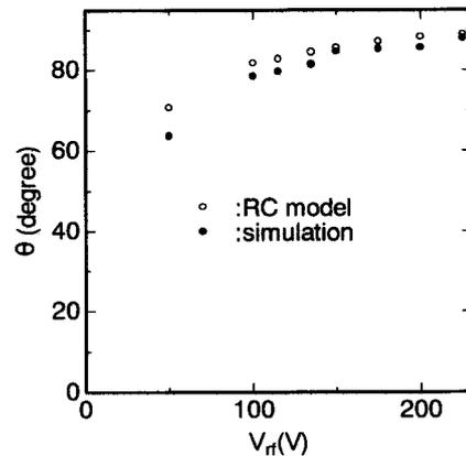
Fig. 6 The dependence of the phase angle difference on the RF voltage (parameters are the same as Fig. 3).
