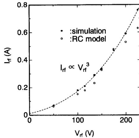
Fig. 5 The dependence of the RF current on the RF voltage (parameters are the same as Fig. 3).
