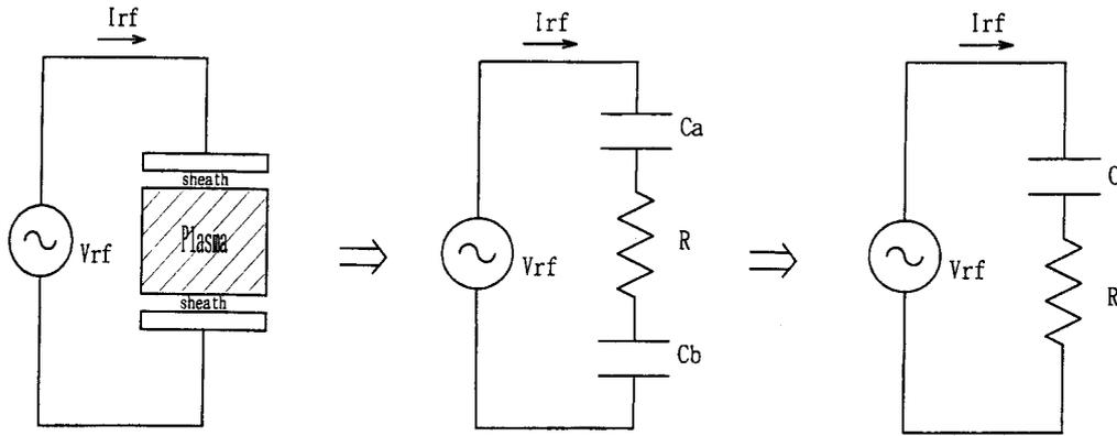
Fig. 1 Equivalent circuit
