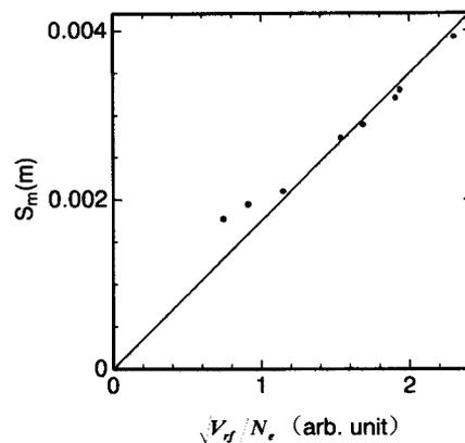
Fig. 7 The variation of the sheath width as function of  $\sqrt{V_{rf}/N_e}$  (parameters are the same as Fig. 3).
