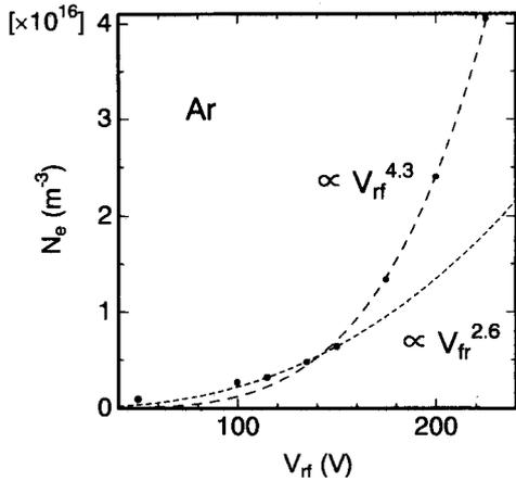
Fig. 4 The dependence of the electron density on the RF voltage (parameters are the same as Fig. 3).
