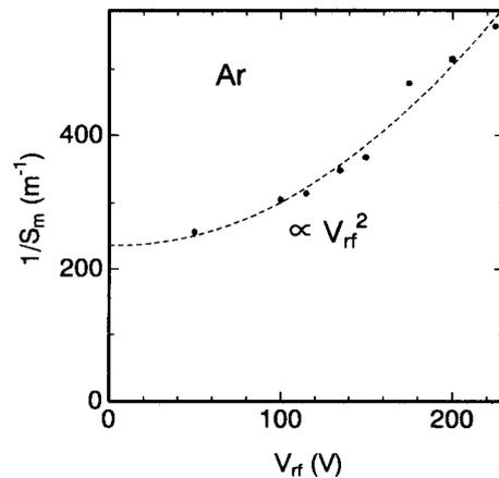
Fig. 3 The dependence of the sheath width on the RF voltage ( $P = 66.5$  Pa,  $L = 0.05$  m and other parameters are given in Table I).
