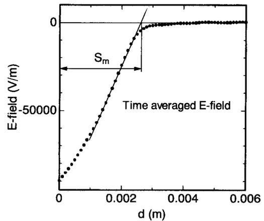
Fig. 2 Time averaged electric field in a sheath ( $V_{rf} = 150$  V,  $P = 66.5$  Pa,  $L = 0.05$  m and other parameters are given in Table I).
