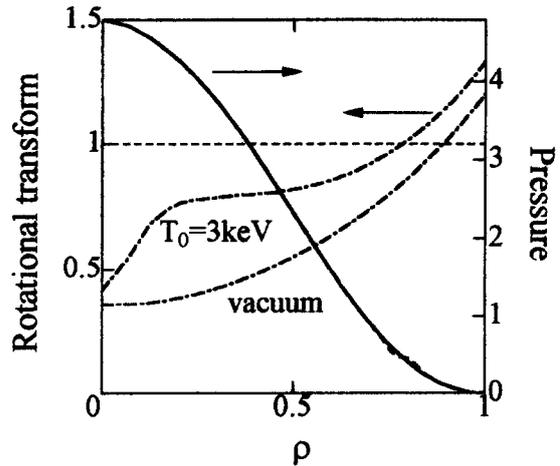
Fig. 4 Profiles of the rotational transform (dashed-dotted lines) for vacuum and  $T_0 = 3$  keV cases and the pressure at  $T_0 = 3$  keV in the standard configuration. Solid and dashed lines show the smooth and the flattened ( $w = 0.02$ ) pressure profiles, respectively.
