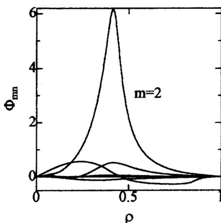
Fig. 3 Fourier components of the stream function of the  $n = 1$  ideal mode at  $\beta(0) = 2\%$  with the smooth pressure profile in the inward-shifted configuration.
