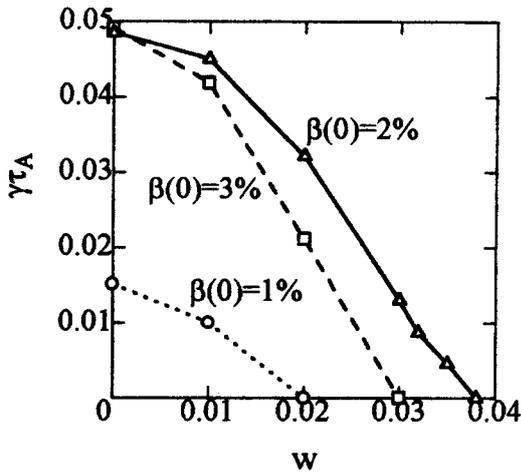
Fig. 2 Growth rate of the  $n = 1$  ideal mode in the inward-shifted configuration at  $\beta(0) = 1, 2$  and  $3\%$  versus the width of the pressure flattened region.
