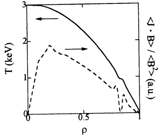
Fig. 5 Profiles of the temperature (solid line) and the bootstrap current density (dashed line) with  $w = 0.02$  in the standard configuration.
