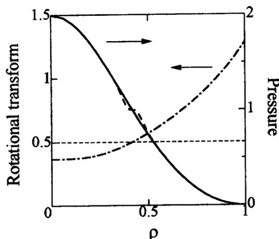
Fig. 1 Profiles of the rotational transform (dashed-dotted line) and the pressure at  $\beta(0) = 2\%$  in the inward-shifted configuration. Solid and dashed lines show the smooth and the flattened ( $w = 0.035$ ) pressure profiles, respectively.
