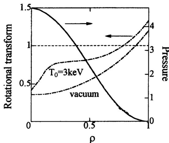
Fig. 4 Profiles of the rotational transform (dashed-dotted lines) for vacuum and  $T_0 = 3$  keV cases and the pressure at  $T_0 = 3$  keV in the standard configuration. Solid and dashed lines show the smooth and the flattened ( $w = 0.02$ ) pressure profiles, respectively.
