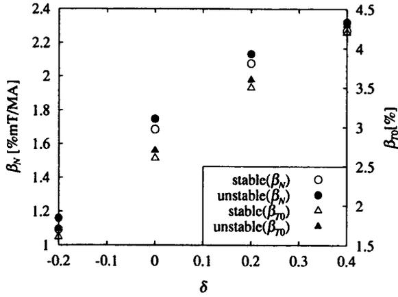
Fig. 3 Dependence of beta limit on triangularity  $\delta$  for the equilibria with  $A = 3$ ,  $\kappa = 1.6$ , and  $q$  profile with  $q_0 = 5.35$  in Fig. 1.
