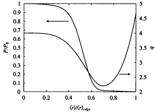
Fig. 6 Pressure and  $q$  profiles for a model of JT-60U reversed shear configuration.
