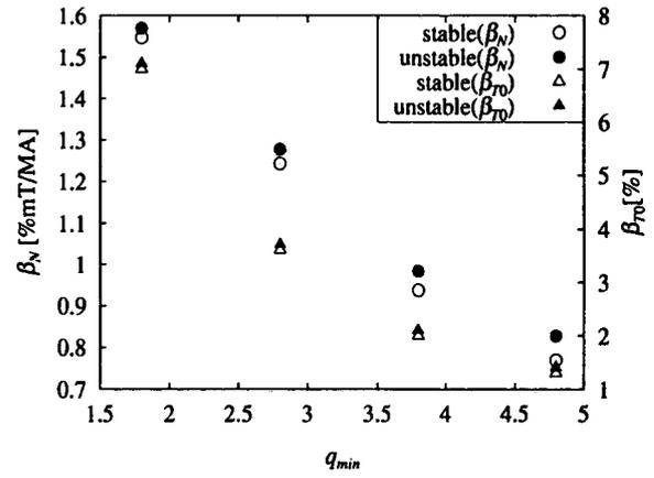
Fig. 5 Dependence of beta limit on  $q_{min}$  for the equilibria with  $A = 3$ ,  $\kappa = 1.8$ ,  $\delta = 0.4$  and  $q$  profiles in Fig. 4.
