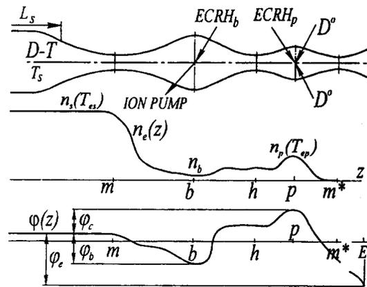
Fig. 1 The scheme of double end mirrors,  $n_e(z)$  and  $j(z)$  are longitudinal distributions of the plasma density and potential,  $L_s$  is the solenoid length.
