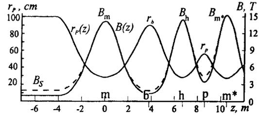
Fig. 3 The plasma radius  $r_p(z)$  and magnetic fields  $\bar{B}(z)$  (solid curve) and  $B_v(z)$  (dashed curve).
