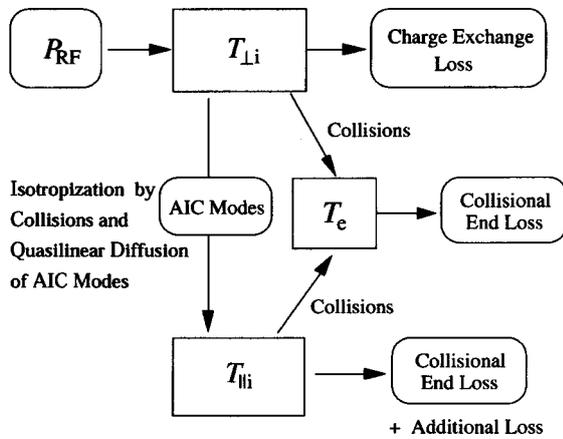
Fig. 1 Power flow chart in the present model for the hot-ion-mode experiment of GAMMA 10.
