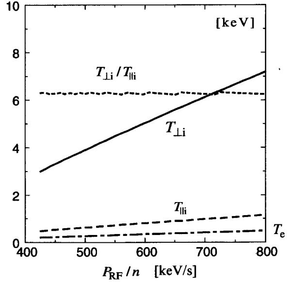
Fig. 3 Ion and electron temperatures as a function of the ICRF power  $P_{RF}/n$  for  $\tau_{ad} = \infty$  and  $W = 0$ .  $T_{\perp i}/T_{\parallel i} \approx 6$  and  $T_{\parallel i}/T_e \approx 2$  for  $T_{\perp i} \approx 3 - 7$  keV.
