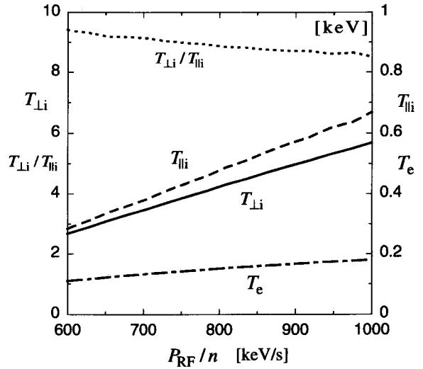
Fig. 2 Ion and electron temperatures as a function of the ICRF power  $P_{RF}/n$  for  $\tau_{ad} = 4$  ms and  $W/n = 10^{-4}$  keV.  $T_{\perp i}/T_{\parallel i} \approx 9$  and  $T_{\parallel i}/T_e \approx 3$  for  $T_{\perp i} \approx 3 - 6$  keV.
