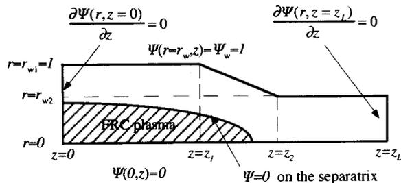
Fig. 1 The boundary condition for the 2D FRC equilibrium with the end mirror field. The perfectly conducting shell is assumed at the wall position. The mirror field is generated when the condition of  $r_{w1} > r_{w2}$  is satisfied.
