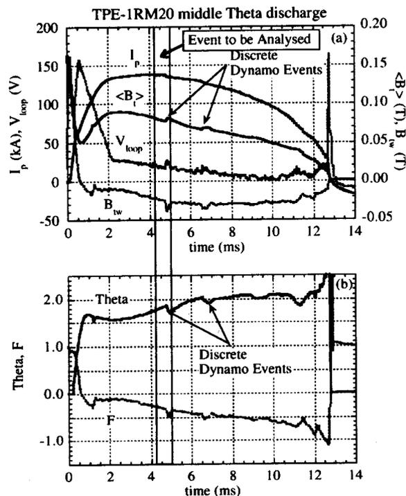
Fig. 1 Typical waveforms of a middle  $\Theta$  discharge in TPE-1RM20 are shown for  $I_p$ ,  $\langle B_t \rangle$  (average toroidal field),  $V_{loop}$  (one turn loop voltage) and  $B_{tw}$  (toroidal magnetic field at the limiter surface) in (a) and  $F$  and  $\Theta$  in (b).
