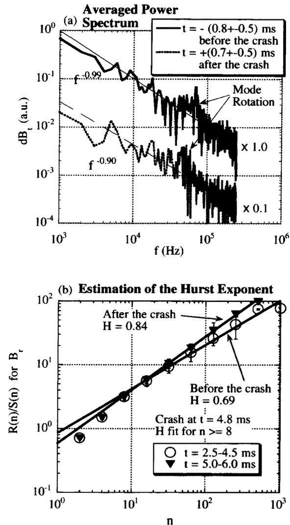
Fig. 3 The magnetic signals of the insertable probe are analyzed. Power spectrum of the  $B_t$  signal in (a) and  $R/S$  versus sampled data for the  $B_t$  signal to estimate the Hurst exponent [5] in (b).
