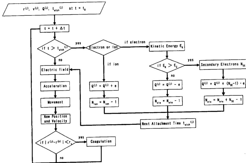
Fig. 1 The flow chart of the simulation procedure
