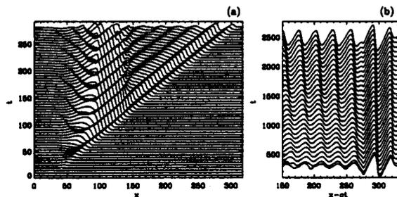
Fig. 2 The electric field in the wake wave in the  $x, t$  plane: a) in the region of plasma inhomogeneity, b) behind the laser pulse.
