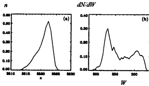
Fig. 4 Distribution function inside the bunch of accelerated electrons versus (a) particle position and (b) particle energy.
