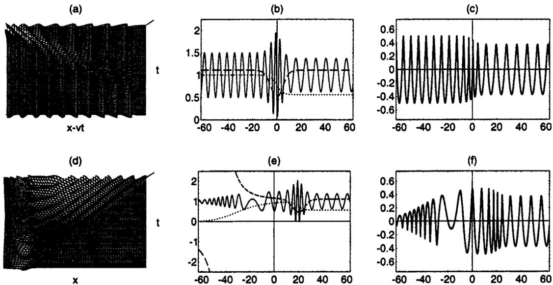
Fig. 1 a) Pattern of the electric field in the wake wave in the  $x - v_y, t$  plane. b) Plasma density distribution (dotted line), dependence of the Jacobian (solid line) and of the wave phase velocity (dashed line) on the Lagrange coordinate. c) Electron momentum versus the Euler coordinate in the breaking wave. d) Pattern of the electric field in the wake wave in the  $x, t$  plane. e-f) The same quantities as in frames (b-c) in the case when the plasma-vacuum interface is taken into account.
