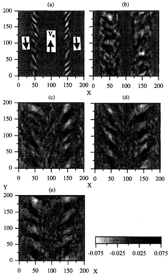
Fig. 1 The time development of the magnetic field  $B_z$ : (a)  $\omega_{pe}t = 14.9$ , (b) 29.8, (c) 44.7, (d) 59.6, (e) 74.5.
