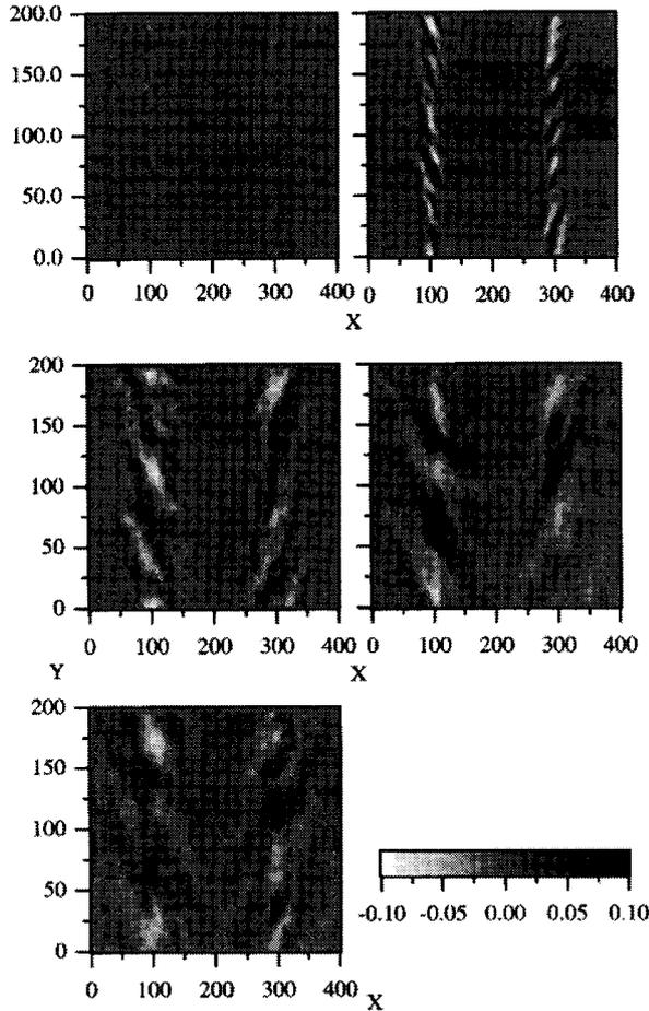
Fig. 3 The time development of the magnetic field  $B_z$ : (a)  $\omega_{pe}t = 14.9$ , (b) 29.8, (c) 44.7, (d) 59.6, (e) 74.5.
