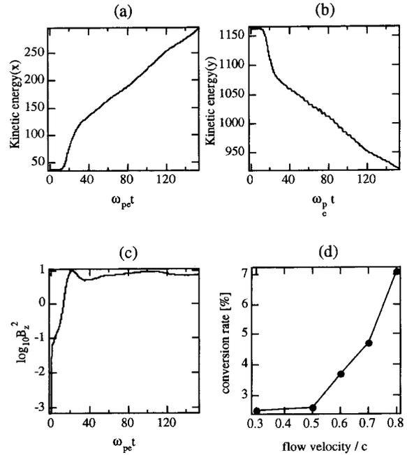
Fig. 2 The time history of the kinetic energy in (a) x-direction, (b) y-direction, and the magnetic field energy (c)  $B_z^2$  and (d) the energy conversion rate.
