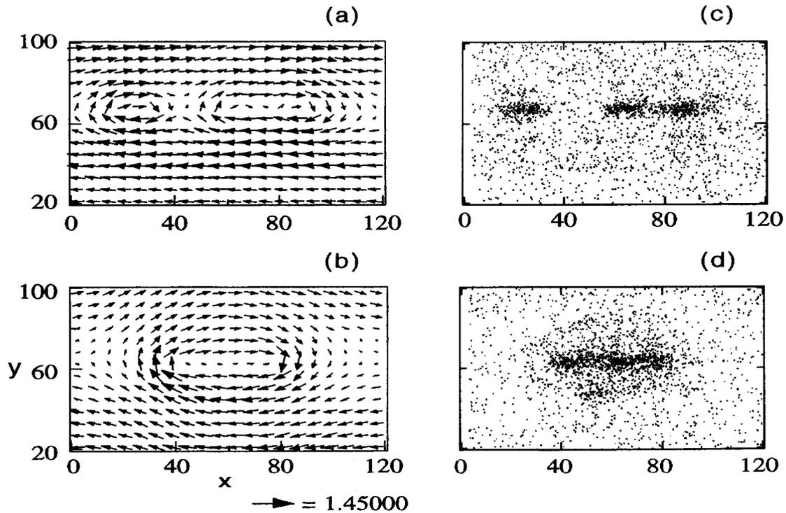
Fig. 1 For a thin current sheet with a width of electron skin depth, the vector plots of the magnetic field  $B_x - B_y$  at (a)  $\omega_{pe}t = 21.08$  and (b)  $\omega_{pe}t = 31.62$  in the  $x$ - $y$  plane. The electron spatial distribution at (c)  $\omega_{pe}t = 21.08$  and (d)  $\omega_{pe}t = 31.62$  in the  $x$ - $y$  plane.
