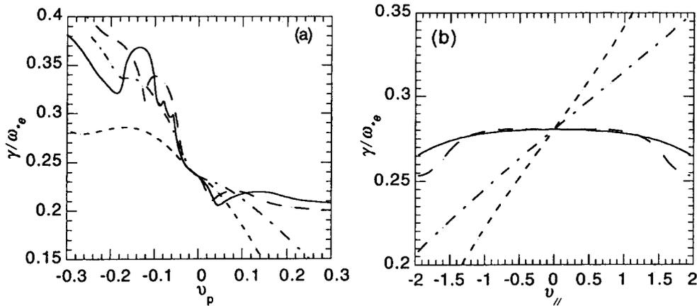
Fig. 2 Normalized growth rate of the global branch versus perpendicular (a) and parallel (b) rotation velocity profile in the weak magnetic shear region. The corresponding curves and parameters are the same as in Fig. 1 except  $L_B = 50$ ,  $L_s \rightarrow \infty$ ,  $k_z = 0.005$ .
