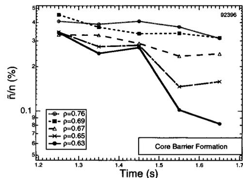
Fig. 1 Fluctuation amplitude at several spatial locations before and after the formation of a core transport barrier showing rapid drop in turbulence inside of  $\rho = 0.65$ . Outside of the region, there is little change in the fluctuation amplitude. Broadband density fluctuations are integrated over the range 80 to 350 KHz.
