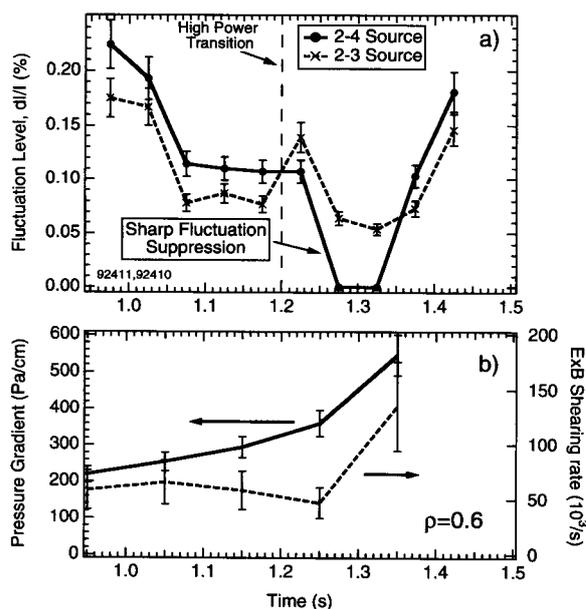
Fig. 3 (a) Comparison of the fluctuation amplitude in two discharges at  $\rho = 0.6$  with initially similar conditions, one with a two to three source transition, and one with a two to four source transition. (b) Pressure gradient and  $E \times B$  shearing rate evolution at the same minor radius.
