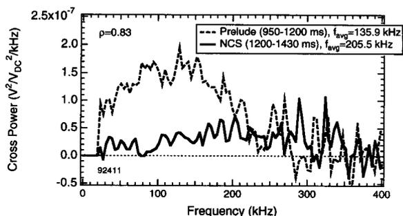
Fig. 2 Broadband density fluctuation spectrum before and after the formation of an internal transport barrier showing the reduction in amplitude due to the barrier formation and increase in the average frequency from the increasing doppler shift.
