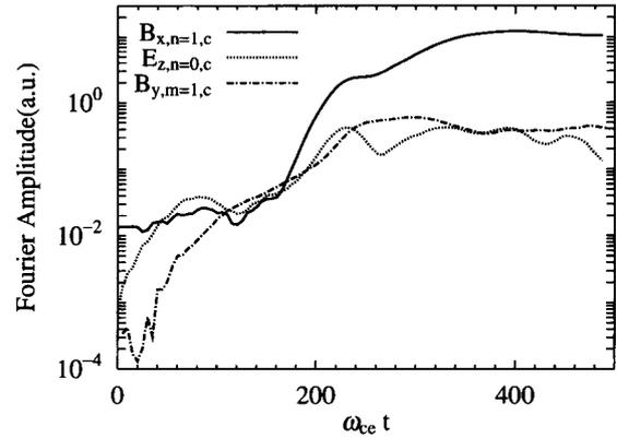
Fig. 3 Temporal evolutions of the Fourier modes for the case of  $E_0 = 0.02B_0$  where the solid, dashed, dotted, and dot-dashed lines represent the  $n = 1$  mode of  $B_x(0,0,z)$ , the  $n = 0$  mode of  $E_z(0,0,z)$ , and the  $m = 1$  mode of  $B_y(x,0,0)$ , respectively. Here,  $m$  stands for the Fourier mode number along the  $x$  axis.
