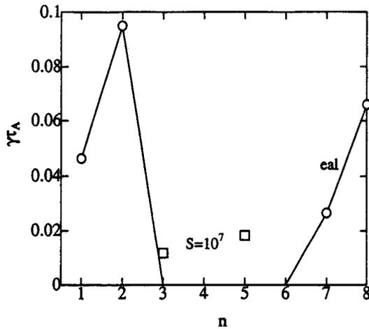
Fig. 3 Growth rates for interchange modes with  $1 \leq n \leq 8$  in a negative shear tokamak. For  $n = 3$  and  $n = 5$ , only the resistive interchange mode becomes unstable and growth rate for  $S = 10^7$  is shown. For  $n = 1, 2, 7$  and  $8$ , the non-resonant ideal mode becomes unstable.
