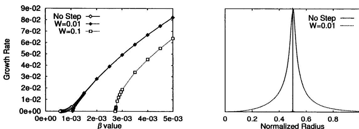
Fig. 2 Growth rate of  $m = 2/n = 1$  mode is shown as a function of  $\beta(0)$  for a cylindrical plasma with rotational profile of  $\iota(r) = 0.4 + 0.2r^2$  in the left hand side figure. Eigenfunctions for  $W = 0$  and  $W = 0.01$  at nearly marginal state are plotted in the right hand side figure.
