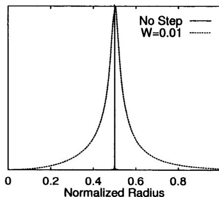
Fig. 2 Growth rate of  $m = 2/n = 1$  mode is shown as a function of  $\beta(0)$  for a cylindrical plasma with rotational profile of  $\iota(r) = 0.4 + 0.2 r^2$  in the left hand side figure. Eigenfunctions for  $W = 0$  and  $W = 0.01$  at nearly marginal state are plotted in the right hand side figure.
