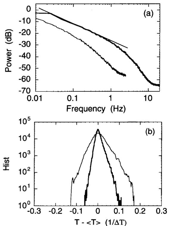
Fig. 2 (a) Power spectra of the temperature fluctuations. (b) Histograms of the temperature fluctuations. Thin line:  $Ra = 1.85 \times 10^9$ . Thick line:  $Ra = 5.14 \times 10^{10}$ .
