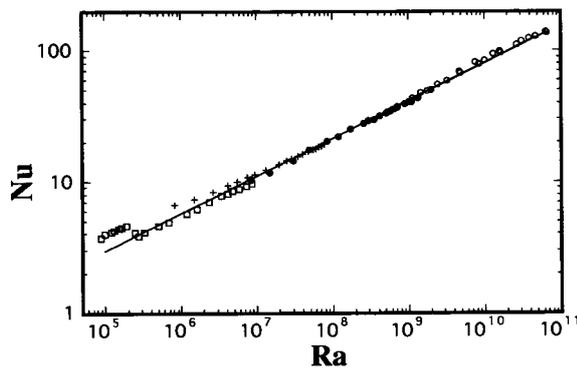
Fig. 1 Nusselt number as a function of Rayleigh number for: circles, large aspect ratio one half cell; crosses, small aspect ratio 1 cell; squares small aspect ratio two cell; bullets, small aspect ratio one half cell. The solid line is  $Nu \sim Ra^{0.295}$ . The discontinuity in the small aspect ratio two data is a result of a pattern competition instability. The reduced slope for small  $Ra$  for the aspect ratio one data results from strong bulk circulation.
