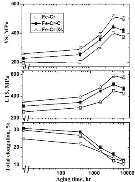
Fig. 1 Evolution of yield stress, ultimate tensile stress and elongation during aging at 475°C.
