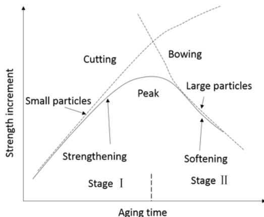
Fig. 8 Age-hardening curve and sketch diagram for precipitation hardening mechanism.
