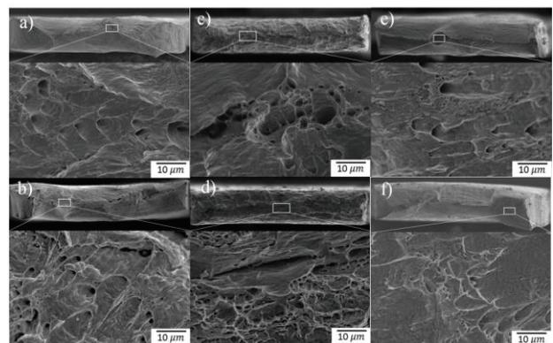
Fig. 3 Ruptured surfaces of the model alloys: a) Fe-Cr, unaged; b) Fe-Cr, aged for 10,000 h; c) Fe-Cr-C, unaged; d) Fe-Cr-C, aged for 10,000 h; e) Fe-Cr-Xs, unaged; f) Fe-Cr-Xs, aged for 10,000 h.
