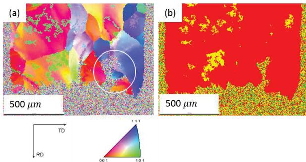
Fig. 5 Fe-Cr-Xs alloy after aged for 5000 h: (a) grain morphology of the ruptured region; (b) phase characterization, ferrite (red color) and martensite (yellow).
