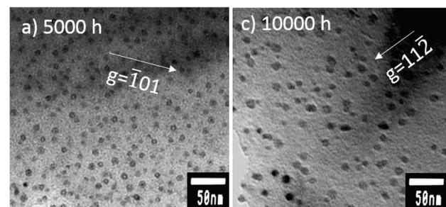
Fig. 7 TEM bright field images of a) Fe-Cr, aged for 5000 h, b) Fe-Cr, aged for 10,000 h.
