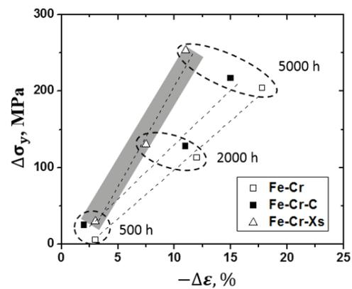
Fig. 2 Linear relations between the change in yield stress,  $\Delta\sigma_y$ , and the change in elongation,  $-\Delta\epsilon$ , of each alloy.
