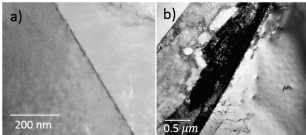
Fig. 4 TEM bright field images of a) Fe-Cr alloy, unaged, b) Fe-Cr-Xs alloy, unaged.
