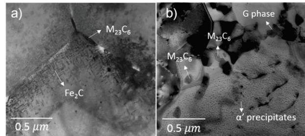
Fig. 6 TEM bright field images of a) Fe-Cr-C alloy, aged for 500 h, b) Fe-Cr-Xs alloy, aged for 5000 h.
