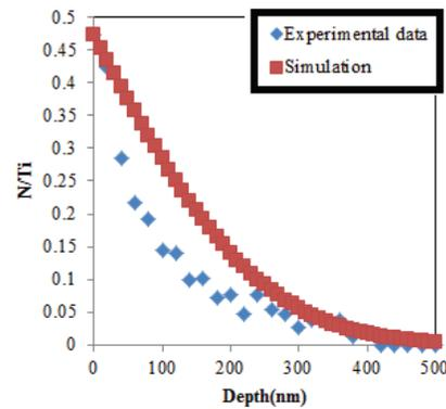
Fig.5 XPS analysis of the titanium plate comparing with a simulation.
