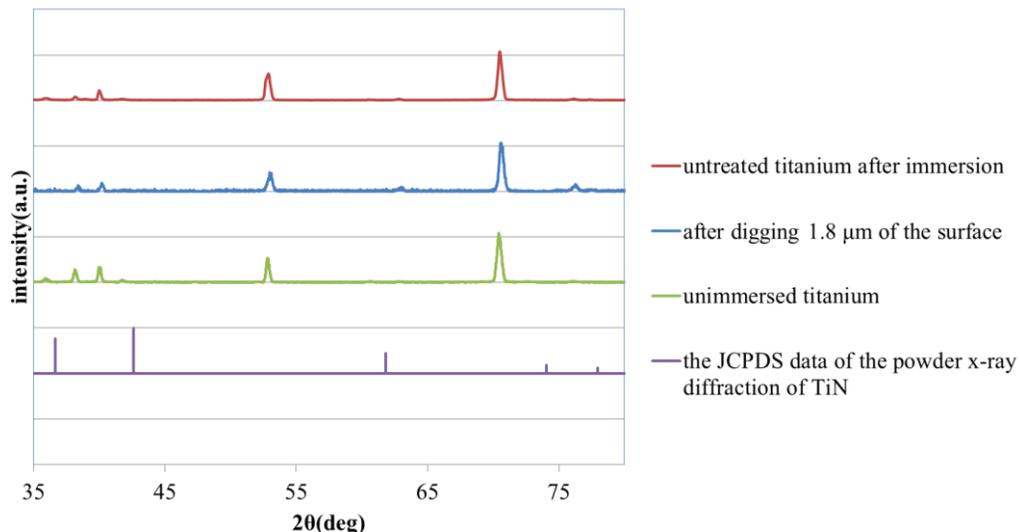
Fig.4 XRD analysis of the titanium plates
