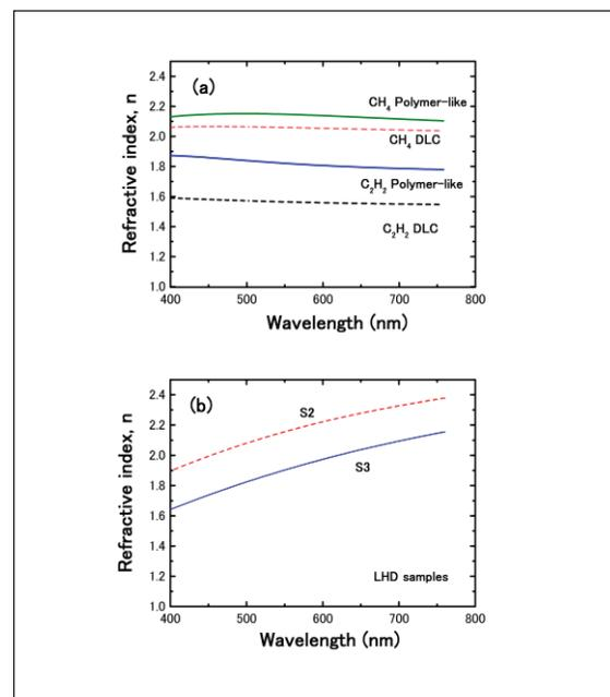
Figure 4. Refractive index measured by the the ellipsometry analysis (a) for reference data using known materials, (b) for LHD samples, S2 and S3.
