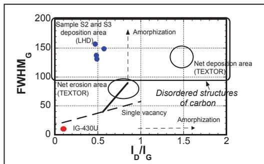
Figure 3. Analytical data of Raman spectroscopy for deposition layers on S2 and S3 samples of LHD (this work), IG-430U graphite target (this work) and deposition and erosion areas on graphite limiter of TEXTOR [11].
