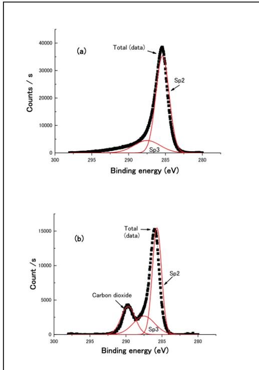
Figure 2. Narrow profile of C1s peak by XPS at (a) a depth of 31.8nm on sample S2 and (b) a depth of 4.5 nm on sample S3. A fitting analysis for the separation of sp<sup>2</sup> and sp<sup>3</sup> carbons is performed.
