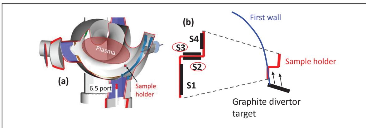
Figure 1. Setups of the sample holder and their location in LHD. (a) The sample holder was installed near the 6.5 port section. (b) The holder has two facings, the sample S2 facing to graphite divertor target and sample S3 facing to the opposite direction of sample S2.
