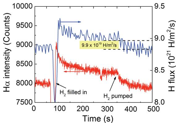
Fig.2 Hydrogen flux and  $\text{H}_\alpha$  signals detected in the upstream hydrogen plasma in VEHICLE-1. Data rearranged from those published in [1].
