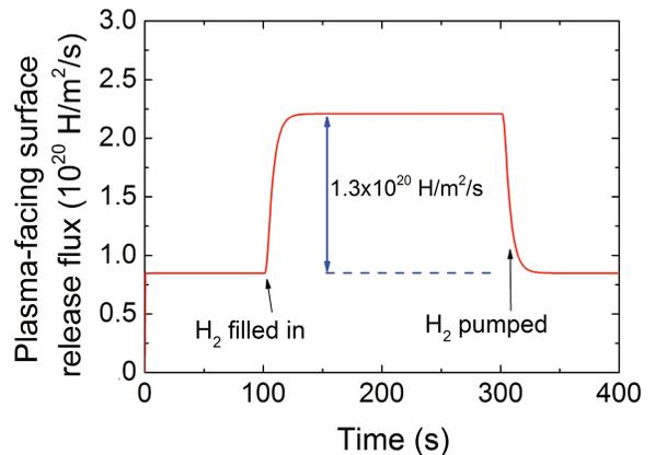
Fig.3 Hydrogen release flux from the plasma facing surface of the  $6 \times 10^{-4}$  m thick membrane predicted by the DIFFUSE code.
