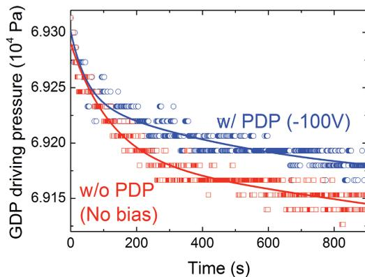
Fig.4 Variation of hydrogen gas pressures measured by an absolute pressure gauge at the PDP downstream side.
