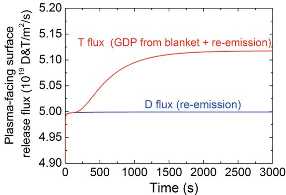
Fig.6 D and T release fluxes at the plasma-facing surface calculated by the DIFFUSE-code for bi-directional PDP-D/T and GDP-T<sub>2</sub>. The total T flux is composed of the re-emission flux of implanted T particle and the GDP-T from the blanket side.
