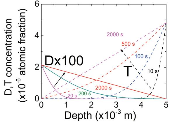
Fig.5 Time evolution of D/T-concentration profiles calculated by the DIFFUSE-code for bi-directional PDP-D/T and GDP-T<sub>2</sub> from the upstream and downstream surfaces, respectively. The D concentration is enlarged by 100 times.
