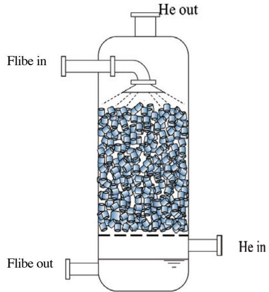
Fig. 5 Overview of He-Flibe counter-current extraction tower
