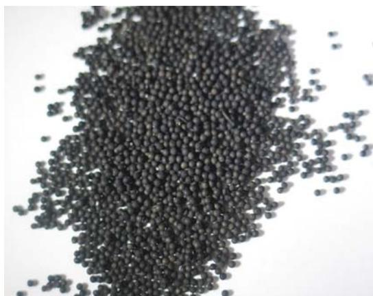
Fig.3 Appearance of 1.0 wt% Pt/ $\text{Li}_4\text{SiO}_4$  pebble
