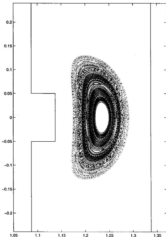
Fig. 3 A double island chain obtained from a self-healed configuration as described in the text. The  $\langle \beta \rangle$  value is 0.2% and the pressure profile is intermediate between the previous two sequences.
