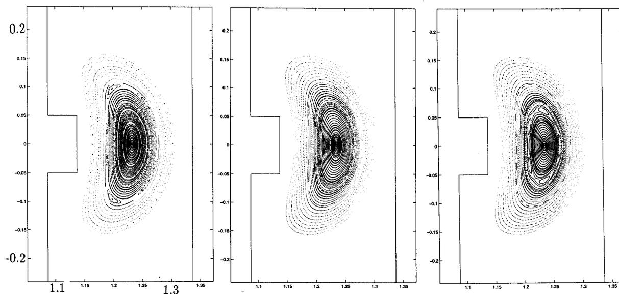
Fig. 1 Flux surface cross-sections from a sequence of equilibria which exhibits self healing as described in the text. From left to right the  $\langle \beta \rangle$  increases from zero to 0.1% to 0.134% with a steep pressure profile inside the island chain. Axis coordinates are in metres from the centre of the device.
