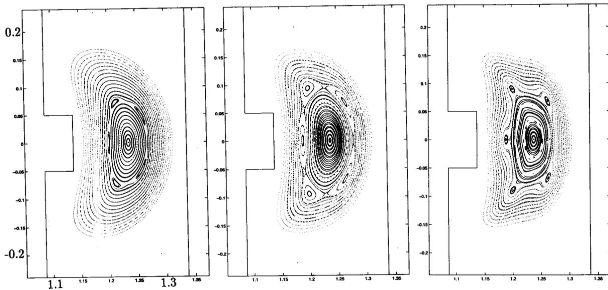
Fig. 2 Flux surface cross-sections from a sequence of equilibria where the 6/5 island chain grows as described in the text. From left to right the  $\langle \beta \rangle$  increases from 0.26% to 0.4% to 0.65% with a broader pressure profile and with additional tuning to control the rotational transform.
