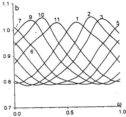
Fig. 2 Distribution of  $B$  over the length of one magnetic field period for magnetic lines, numbered in Fig. 1 for the surface  $\rho_0=12.33$  ( $b=B/B_0$ ,  $\omega = m_p \varphi / 2\pi$ ).
