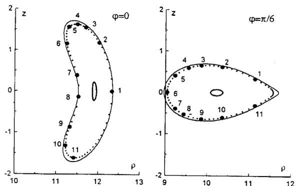
Fig. 1 Boundary surface [6] (solid line) and magnetic surfaces, corresponding to  $\rho_0 = 12.33$  (near boundary,  $t = 1.475$ ) and  $\rho_0 = 11.95$  (inner,  $t = 1.41$ ); the dimensions are given in the same relative units as in [6] ( $\rho_0$  is the initial point of integration in the  $\varphi = 0$  cross-section for  $z = 0$ ).
