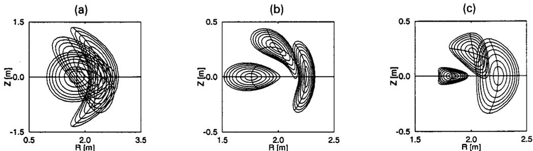
Fig. 2: Magnetic surface cross sections at  $\phi = 0, (1/4)(2\pi/M)$  and  $(1/2)(2\pi/M)$  for (a) QAS, (b) QHS and (c) QBS configurations.
