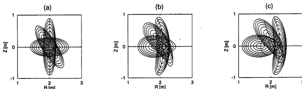
Fig. 1: Magnetic surface cross sections at  $\phi = 0$ ,  $(1/4)(2\pi/M)$  and  $(1/2)(2\pi/M)$  for (a) "Conf.1", (b) "Conf.2" and (c) "Conf.3".
