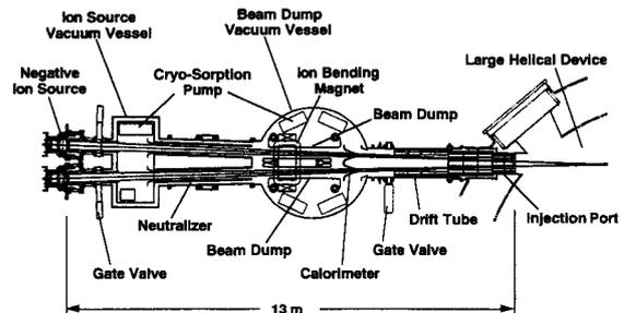
Fig. 3 Schematic diagram of the second beamline (BL2) of the negative-ion-based LHD-NBI system.
