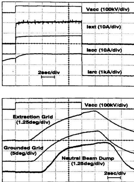
Fig. 2 Example of the time evolution of the acceleration voltage and current, the extraction current, the arc current, and the water temperature rises of the extraction grid, the grounded grid and the neutral beam dump located 13 m downstream, with a prototype LHD-NBI source. The H<sup>-</sup> ion beam power is about 700 kW (73 keV).
