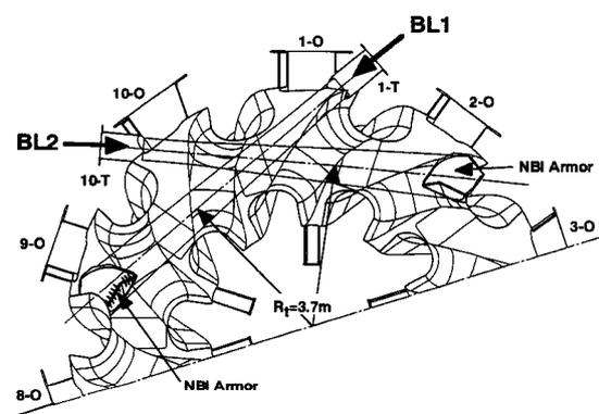
Fig. 1 Schematic diagram of the injected neutral beam path, the location of the injection ports, and the beam facing armors in LHD.
