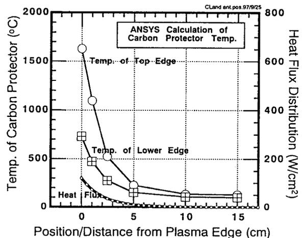
Fig. 7 Calculated temperature increments of the carbon side protector by ANSYS code are shown by changing the top edge position.
