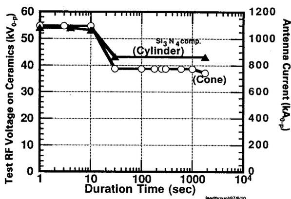
Fig. 1 Successful test records of R&D antenna are plotted. Two kinds of feedthrough were used in the tests.
