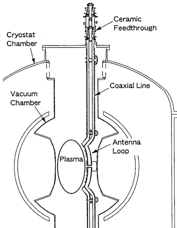
Fig. 3 Cross sectional view of the fast wave ICRF antenna in LHD.
