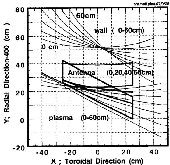
Fig. 5 The horizontal cross sectional cuts of the antenna, the plasma surface and the vacuum chamber wall at the different altitudes.
