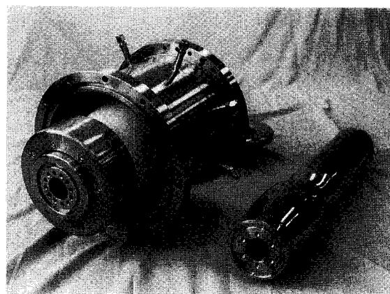
Fig. 2 Photograph of the cone type feedthrough. Gas cooling nozzles are located around the outer conductor.
