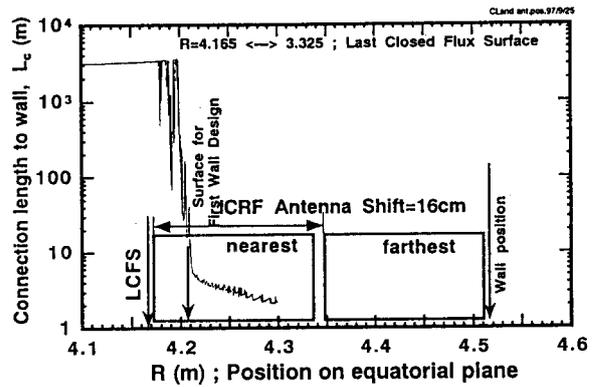
Fig. 4 Antenna moving range is shown in a equatorial plane. The nearest and the farthest positions of antenna are drawn by boxes.
