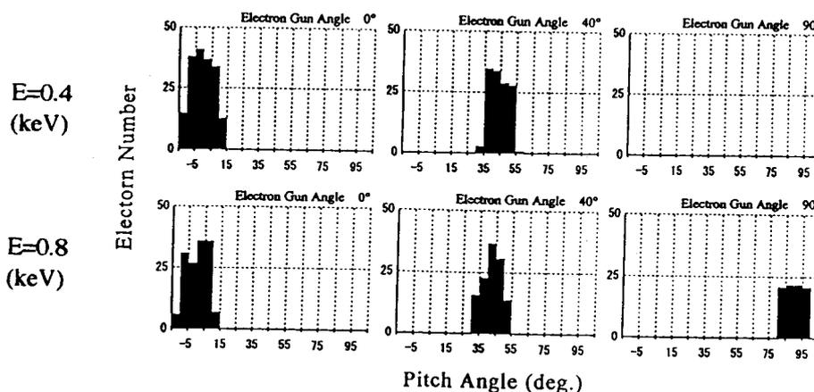
Fig. 5 Relation between electron gun angle and electron pitch angle ( $B = 500$  G, anode diam. = 3 mm).
