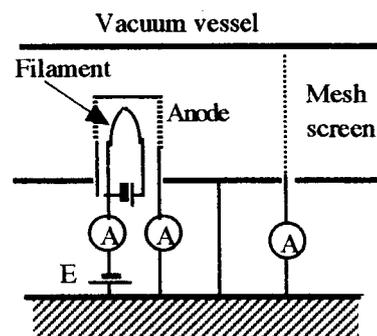
Fig. 1 Principle of stellarator tetrode method for electron confinement study.
