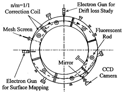
Fig. 2 Experimental set up for magnetic surface and electron confinement studies.
