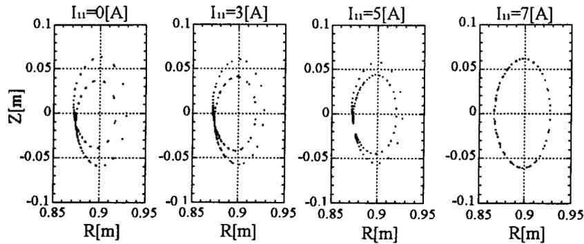
Fig. 3 Computed magnetic surfaces ( $B = 500$  G) under the horizontal earth field of 0.3 G plus  $n/m = 1/1$  helical coil currents  $I_{11}$ .
