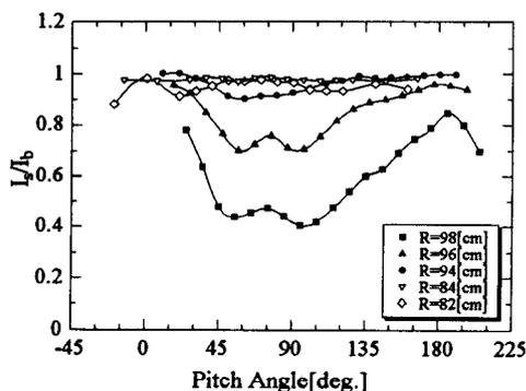
Fig. 6 Normalized screen currents  $I_s/I_B$  versus electron pitch angle for different birth points  $R$ .
