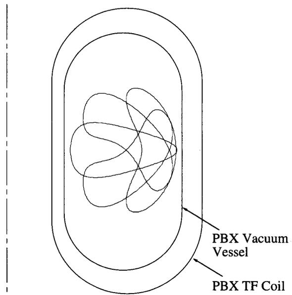
Fig. 3 Cross section showing a number of toroidal cuts of the conducting shell in the PBX-M vacuum vessel.
