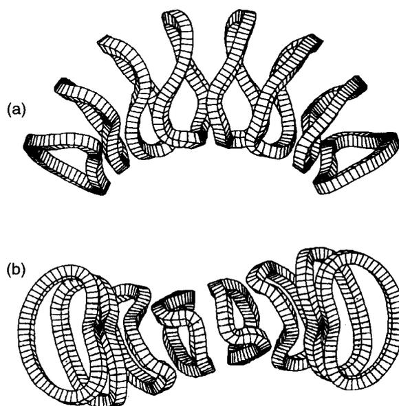
Fig. 1 Modular coils for MHH2 (a) top view (b) side view.
