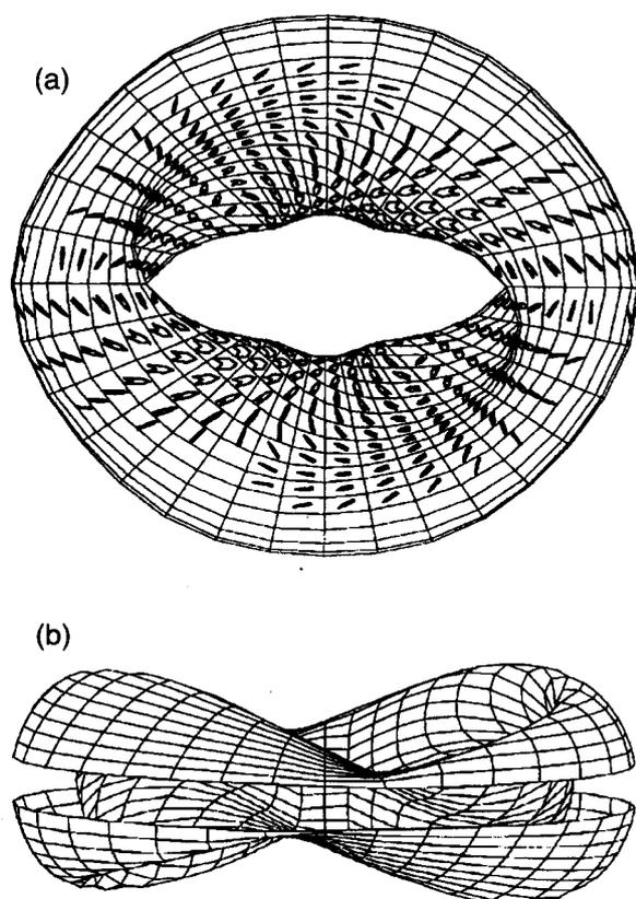
Fig. 4 Conducting shell for MHH2 (a) Showing the eddy current pattern induced by the PBX-M TF, (b) Side view with a 30.5 cm. cut at outboard midplane.
