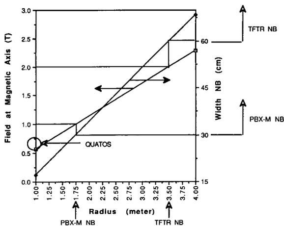
Fig. 2 Scaling of the modular coil design for MHH2.
