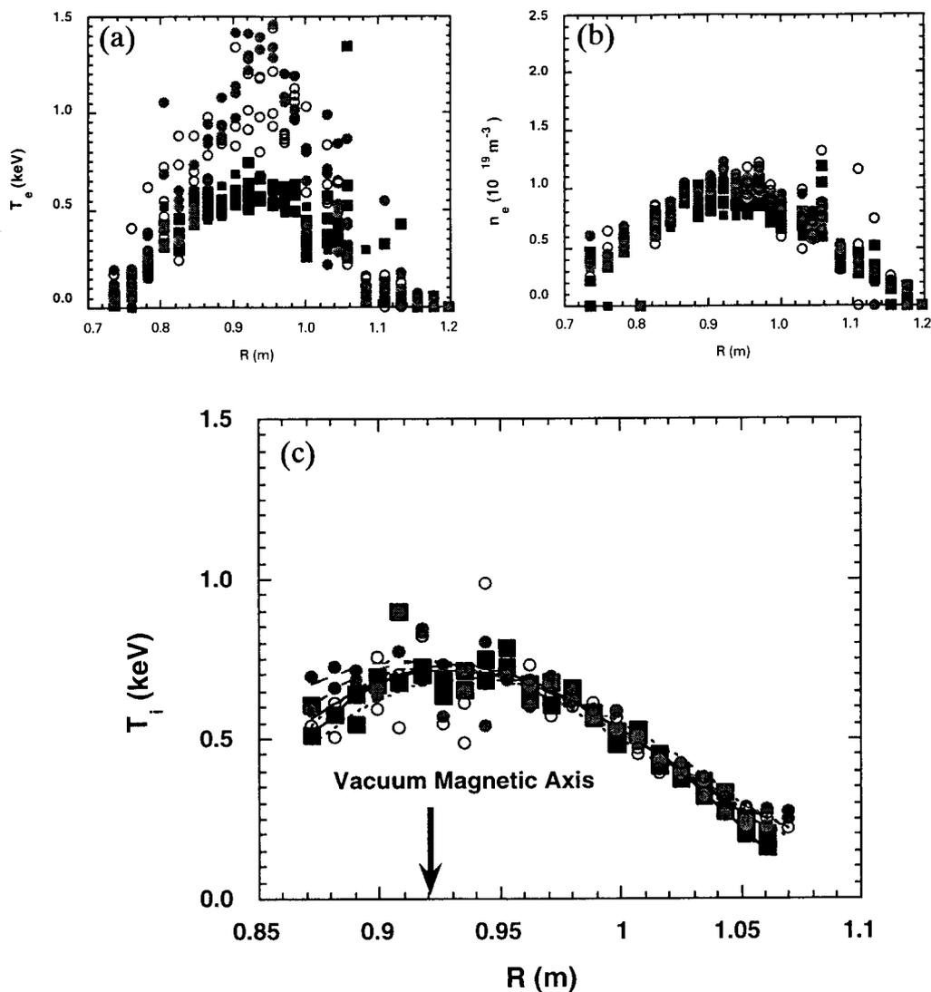
Fig. 2 The profiles of (a) electron temperature, (b) electron density and (c) ion temperature with only NBI#1 injection. The closed square, closed and open circles show the cases without ECH, with on-axis ECH and with off-axis ECH, respectively.
