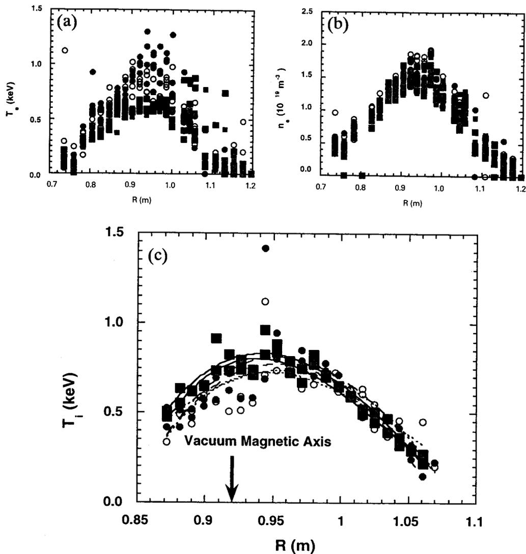
Fig. 3 The profiles of (a) electron temperature, (b) electron density and (c) ion temperature with NBI#1 and NBI#2. The closed square, closed and open circles show the cases without ECH, with on-axis ECH and with off-axis ECH, respectively.
