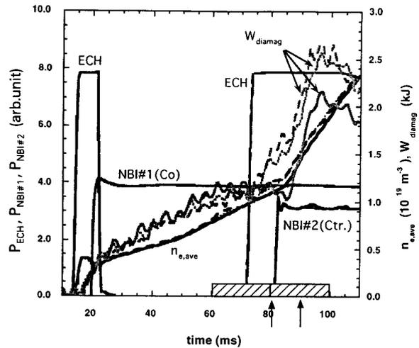
Fig. 1 Time evolution of the heating power, line averaged electron density, stored energy. Thick and broken and dotted line indicates the cases for without ECH, with on-axis ECH, and with off-axis ECH, respectively. The timings of the electron temperature and density profile and ion temperature profiles are shown with arrows and hatched region.
