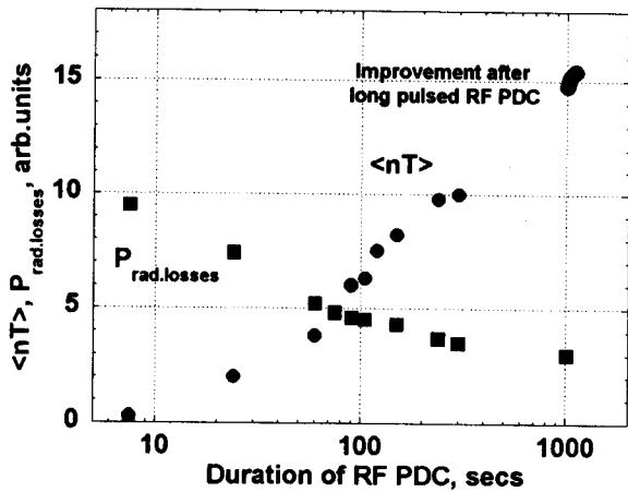
Fig. 3 The dependence of plasma energy (circles) and radiation losses due to light impurities (squares) vs. duration of RF PDC.
