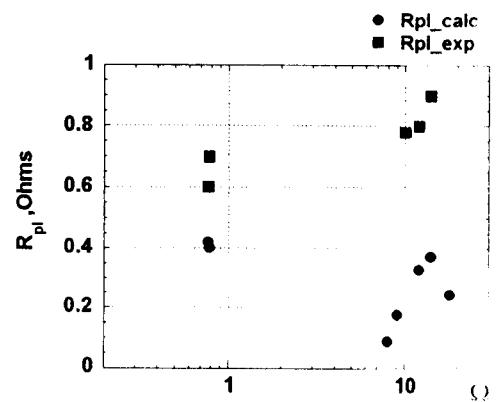
Fig. 4 The comparison of calculated plasma loading resistance values ( $R_{pl, calc}$  - circles) to experimental ones ( $R_{pl, exp}$  - squares) at the different frequencies.
