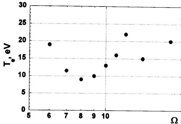
Fig. 2 The dependence of electron temperature vs dimensionless heating frequency  $\Omega \equiv \omega_0 / \omega_{ci}$  in RF PDC.
