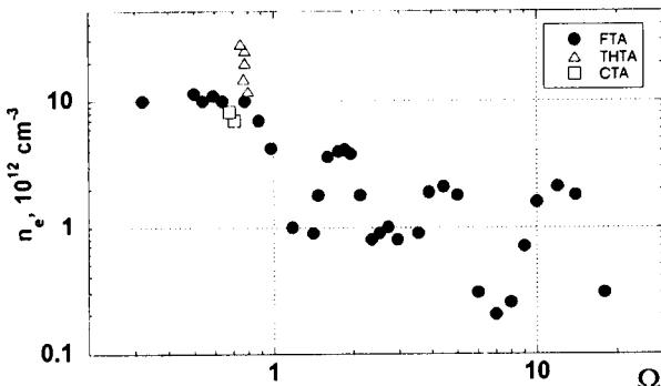
Fig. 1 The dependence of produced plasma density vs. dimensionless heating frequency  $\Omega = \omega_0 / \omega_{ci}$ . The data obtained in experiments with different type of RF antennae (FTA-circles, THTA-triangles, and CTA-squares) is summarized.
