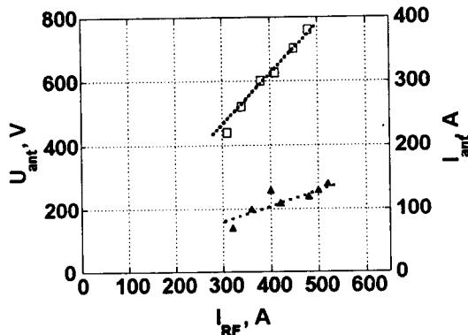
Fig. 5 The dependencies of antenna potential (squares) and rectified current (triangles) onto the RF antenna as a function of RF current in the antenna.
